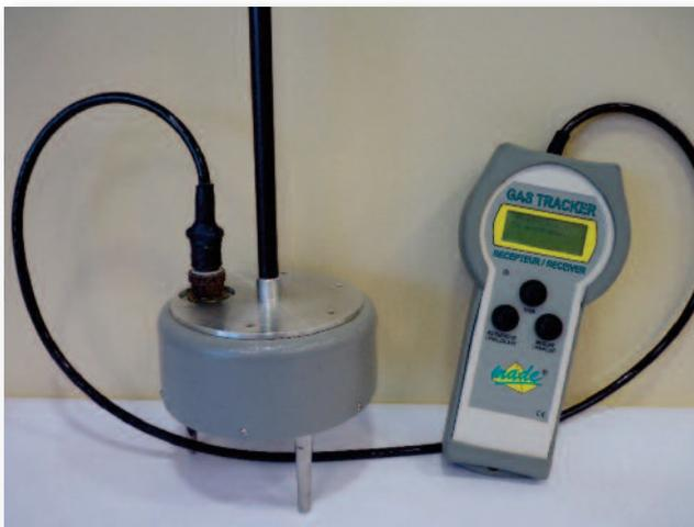
The GasTracker™ receiver, using a listening device placed on the ground and connected to a hand-held receiver, displays the results.
